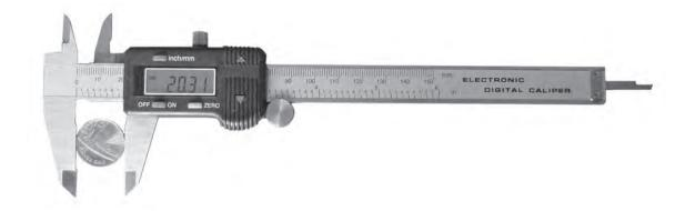
The digital caliper gives readings to the nearest 0.01 mm.
